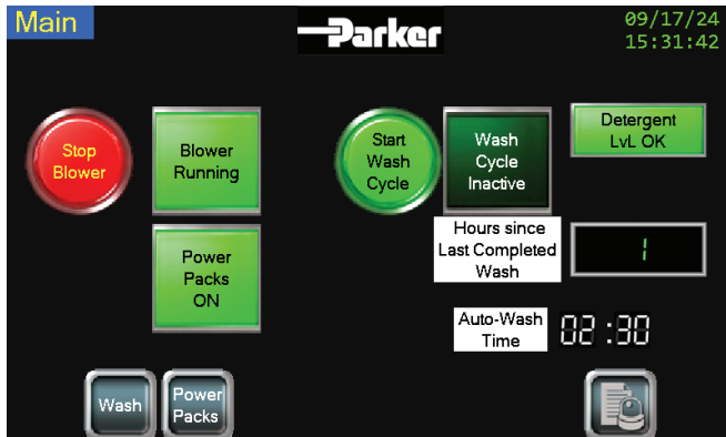
FIGURE 3. Main Operator Screen - Power Packs ON
